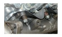
Step 4. Reinstall the factory sensor to the PPE Passenger Side Exhaust Manifold.
